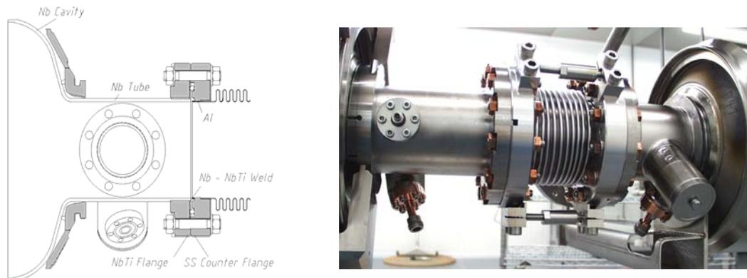
**Figure 7:** Flange design and bellow connection of the TTF cavities using NbTi-flanges and massive aluminum gaskets
