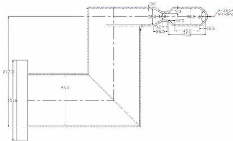
Figure 5.11: Cross section A-A in the pre-dipole vacuum vessel.
