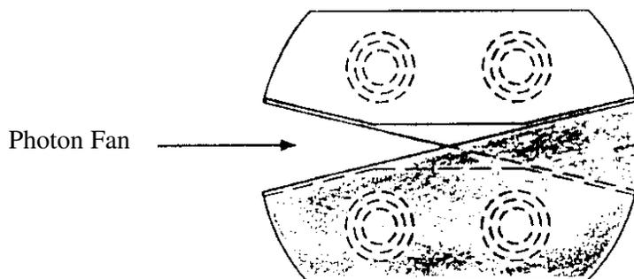
Figure 5.29: Cross section of the crotch absorber.
