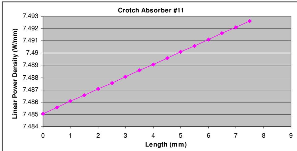
Figure 5.27: Power absorbed by the crotch absorber #11, the overall power is 0.06 kW.
