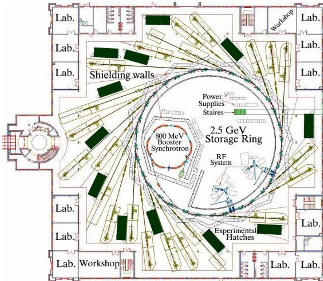
Figure 5.2: An overview of the SESAME machine and experimental hall.
