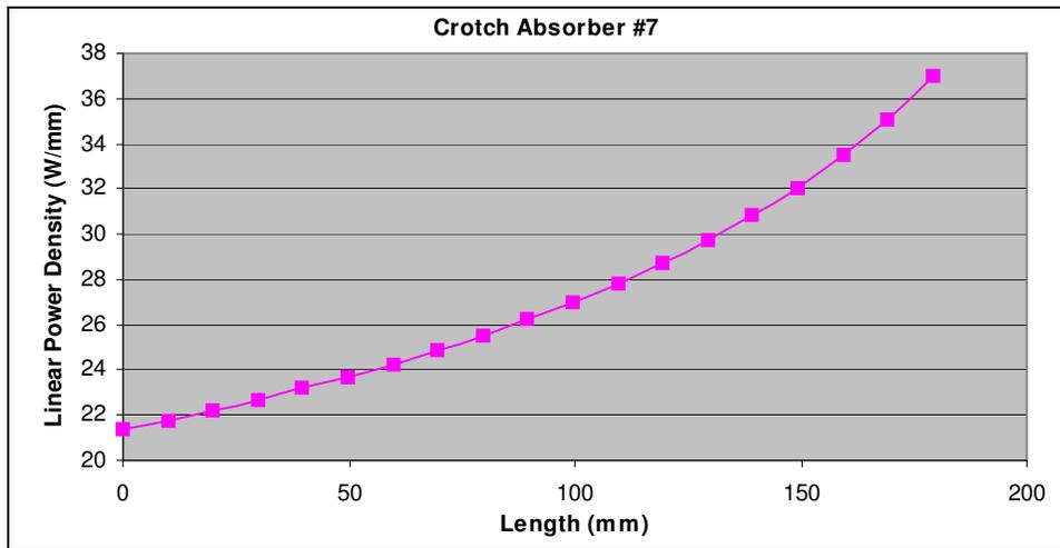
Figure 5.23: Power absorbed by the crotch absorber #7, the overall power is 5.171 kW.
