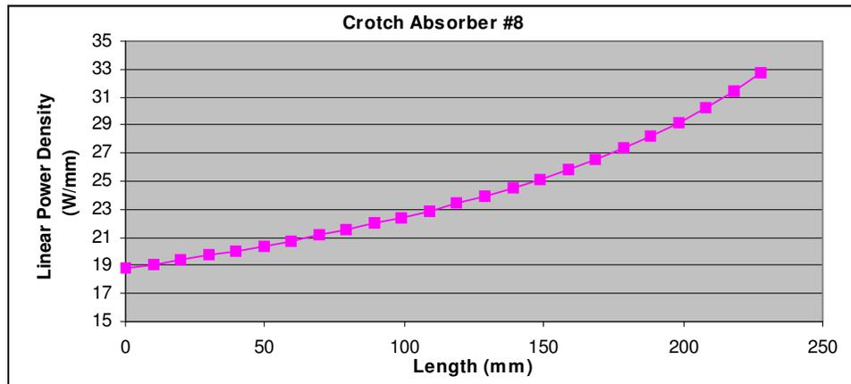
Figure 5.24: Power absorbed by the crotch absorber #8, the overall power is 5.76 kW.
