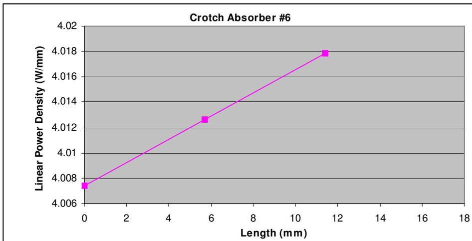
Figure 5.22: Power absorbed by the crotch absorber #6, the overall power is 0.121 kW.
