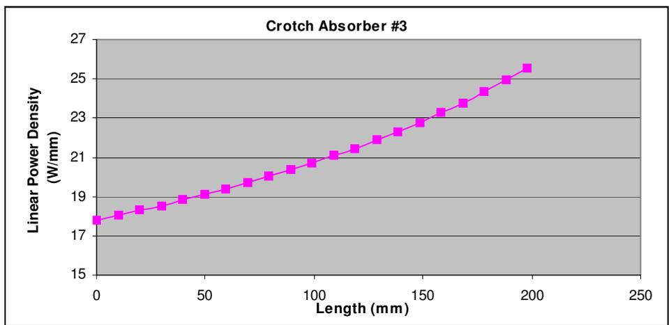
Figure 5.19: Power absorbed by the crotch absorber #3, the overall power is 4.418 kW.
