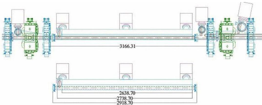
Figure 5.8 The short straight section vacuum vessel.
