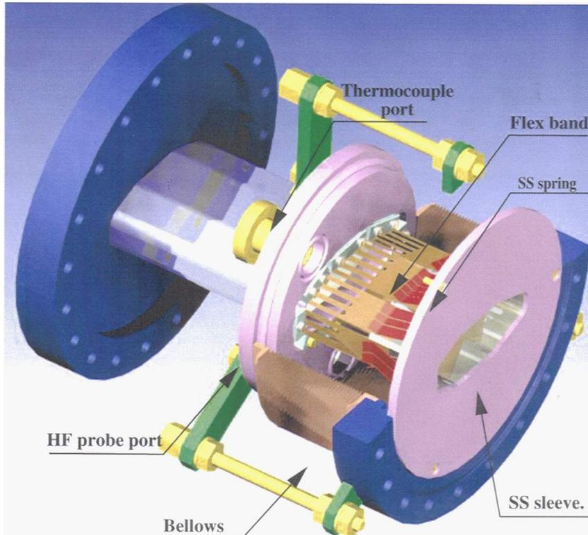
Figure 5.13: Schematic of an RF shielded bellows, SLS/SOLEIL cooperation [3].
