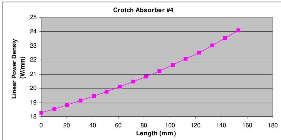
Figure 5.20: Power absorbed by the crotch absorber #4, the overall power is 3.33 kW.
