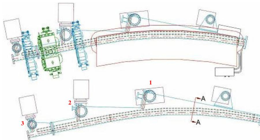
Figure 5.4: The design of the first dipole vacuum chamber in the unit cell (Type 1)
