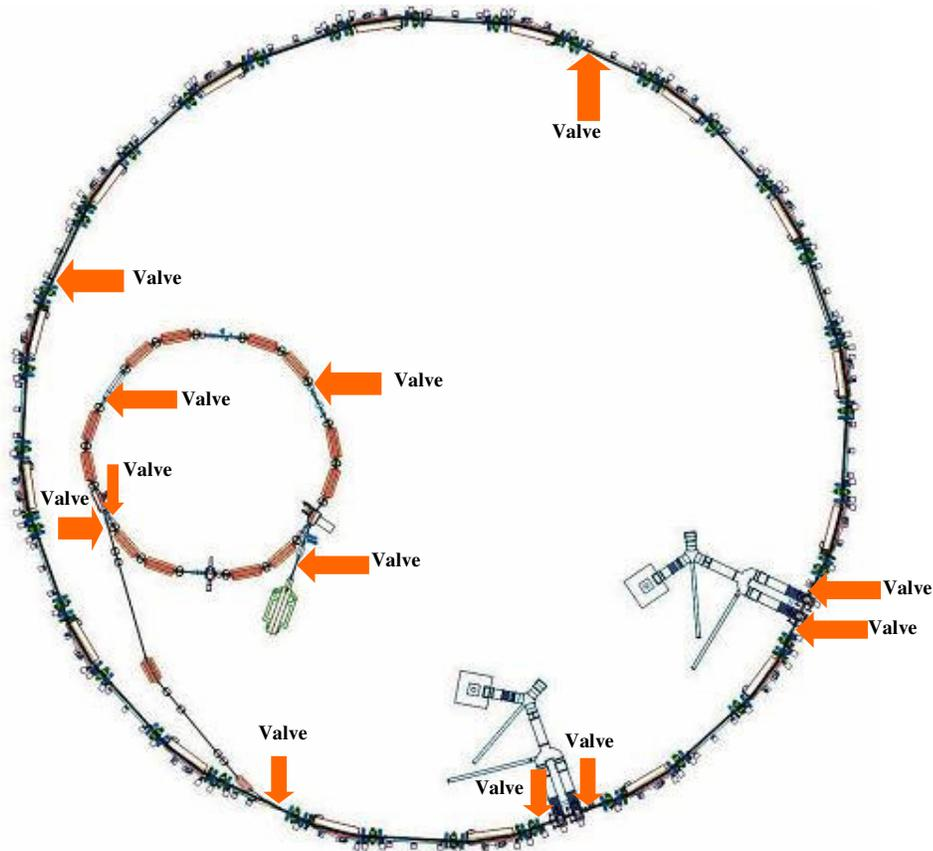
Figure 5.14: the location of the gate valves around the machine.
