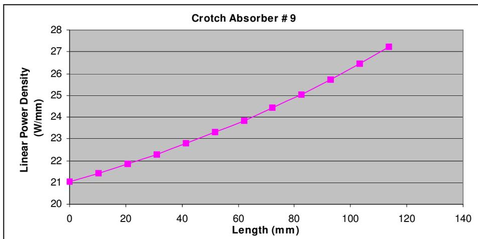
Figure 5.25: Power absorbed by the crotch absorber #9, the overall power is 2.85 kW.
