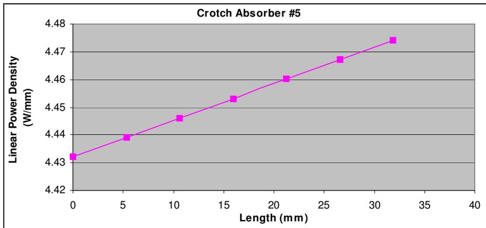
Figure 5.21 Power absorbed by the crotch absorber #5, the overall power is 0.312 kW.
