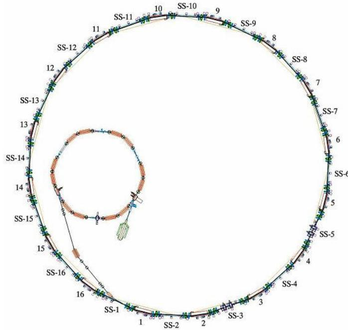
Figure 5.1: the naming system for the SESAME storage ring.
