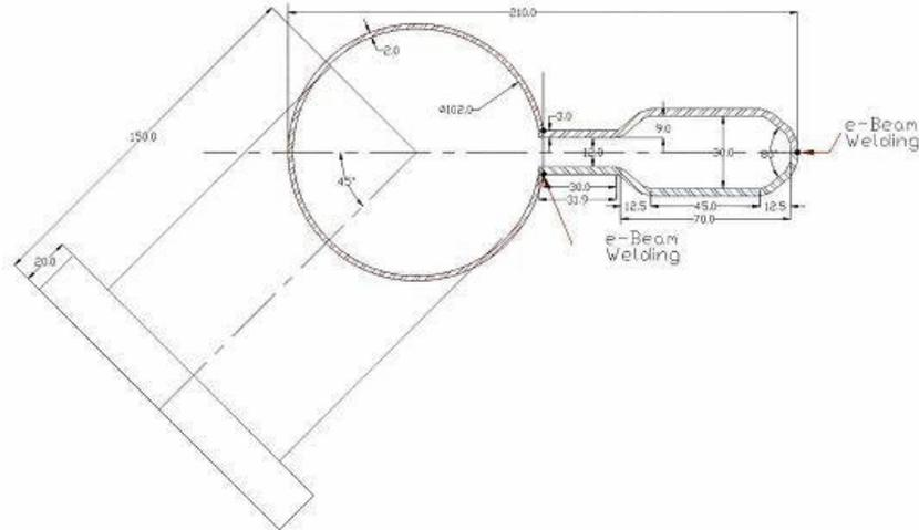
Figure 5.9: Cross section A-A in the straight section vacuum vessel.
