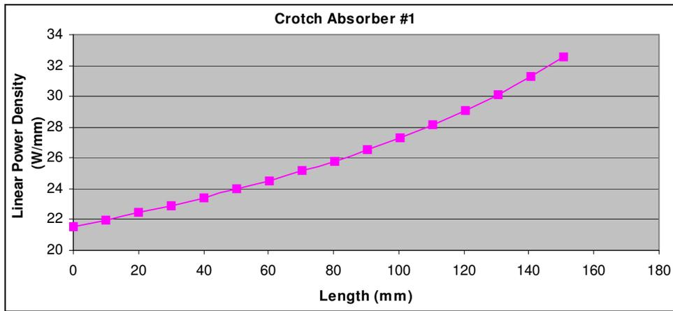
Figure 5.17: Power absorbed by the crotch absorber #1, the overall power is 4.127 kW.
