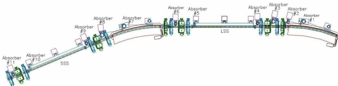
Figure 5.16: The location and the naming of the absorbers in the super period cell of SESAME.
