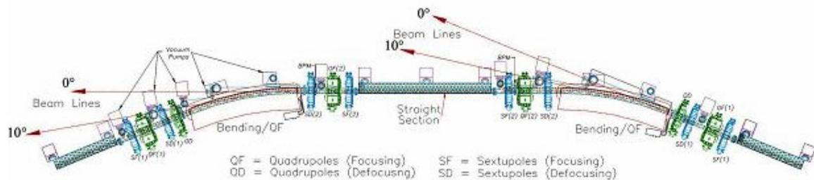
Figure 5.3: The unit cell of the storage ring.
