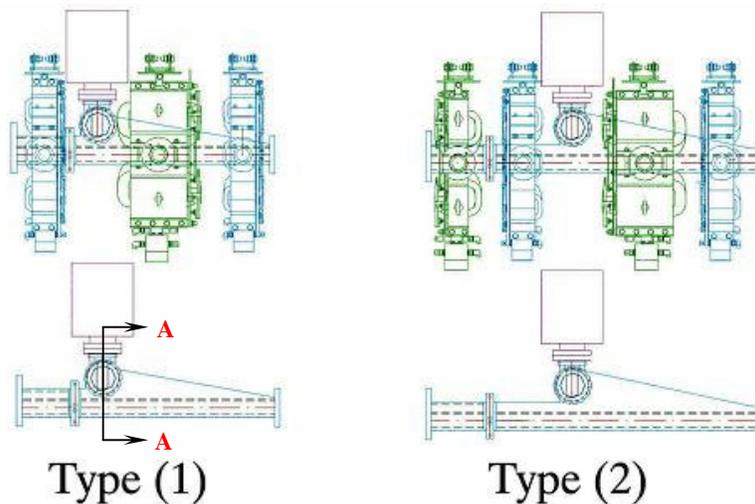
Figure (5.10) the pres-dipole vacuum chamber.
