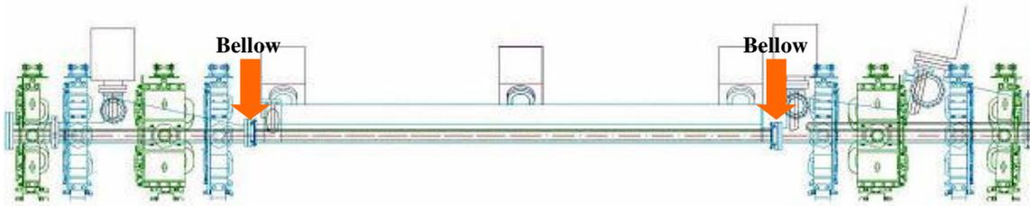
Figure 5.12 The position of the bellows in the straight section.
