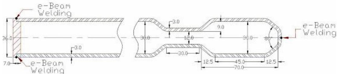
Figure 5.6: Cross section of the dipole vacuum chamber, section A-A.
