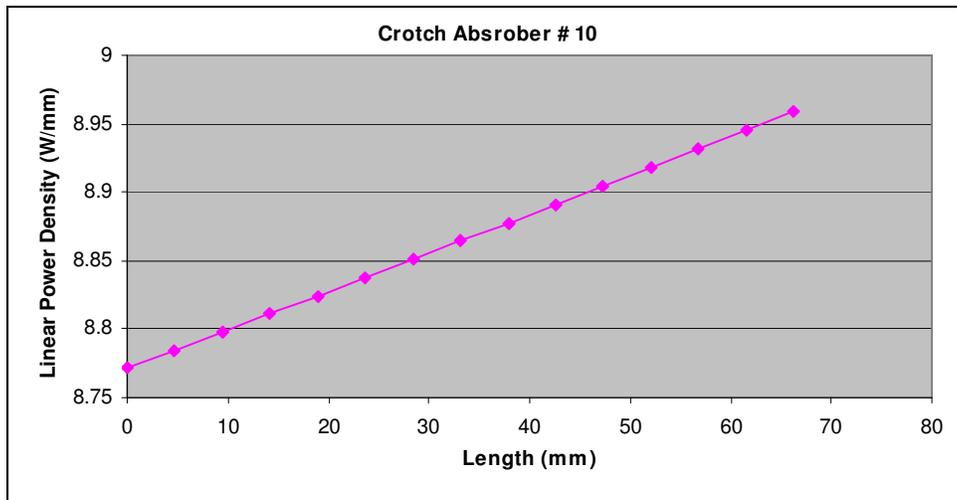
Figure 5.26: Power absorbed by the crotch absorber #10, the overall power is 0.630 kW.
