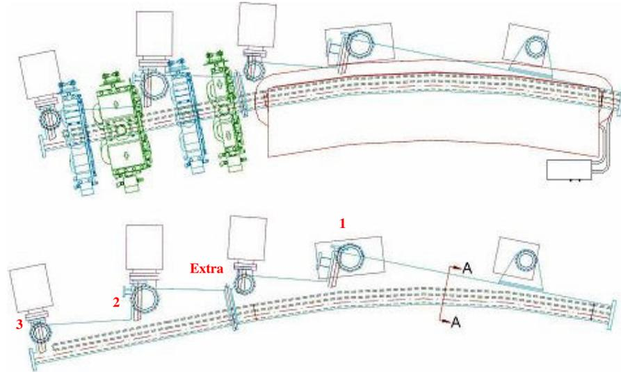
Figure 5.5: The design of the second dipole vacuum chamber in the unit cell (Type 2).
