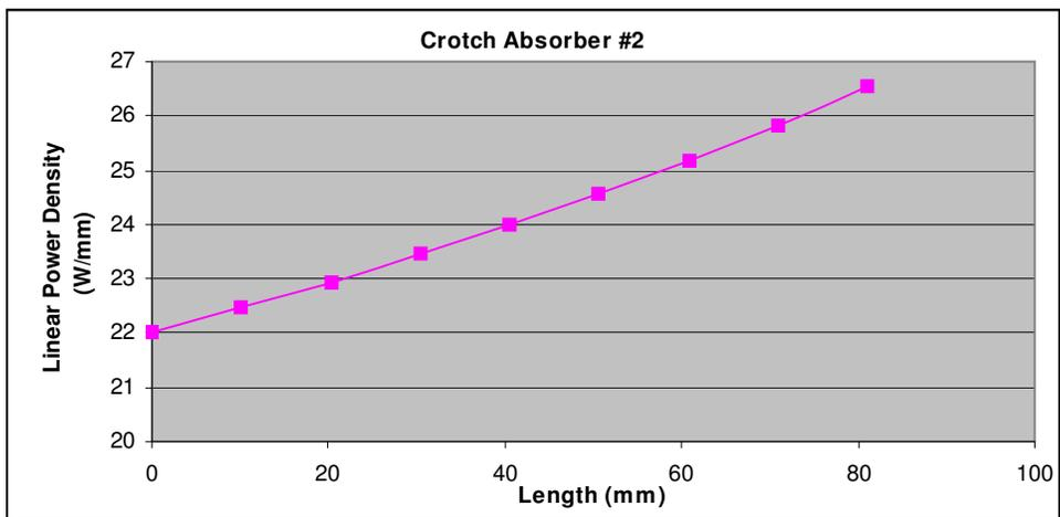
Figure 5.18: Power absorbed by the crotch absorber #2, the overall power is 2.169 kW.
