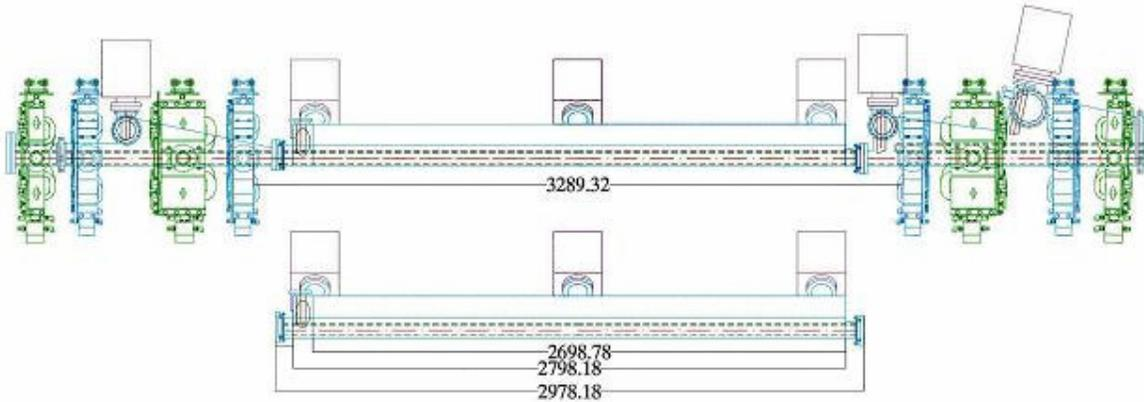
Figure 5.7: The long straight section vacuum vessel.
