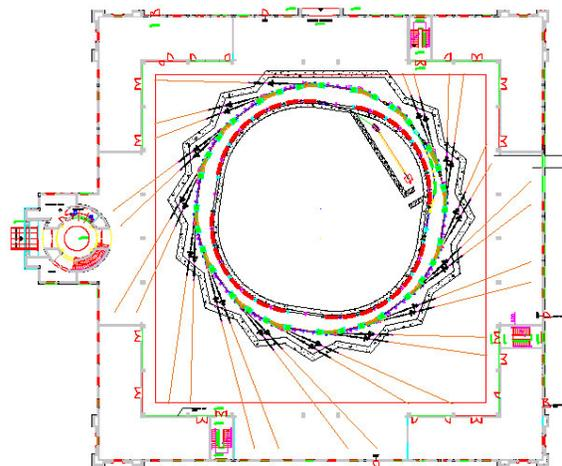
Figure 3: SESAME layout with full-energy injector.
