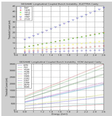
Figure11: Threshold current due to HOM's for ELETTRA type cavity (top) and EU HOM damped cavity (bottom).
