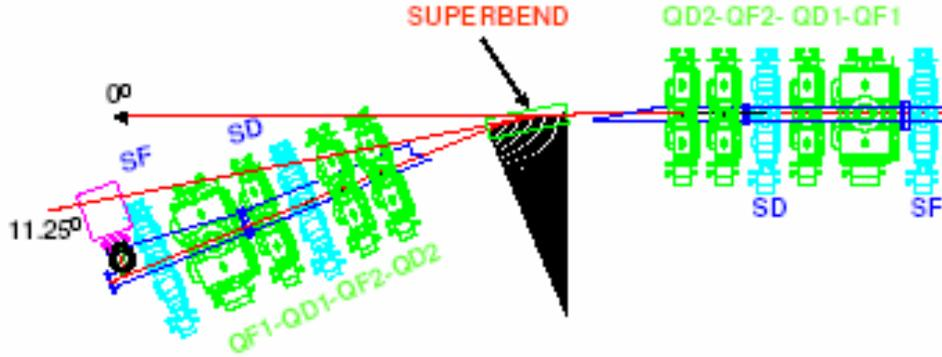
Figure 5: Layout of SUPERBEND solution in SESAME
