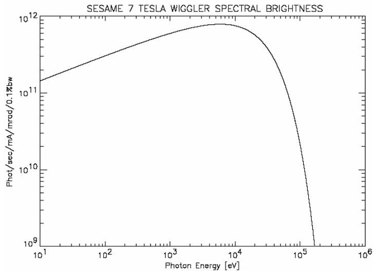
Figure 6: 7T-Wiggler Spectral Brightness.
