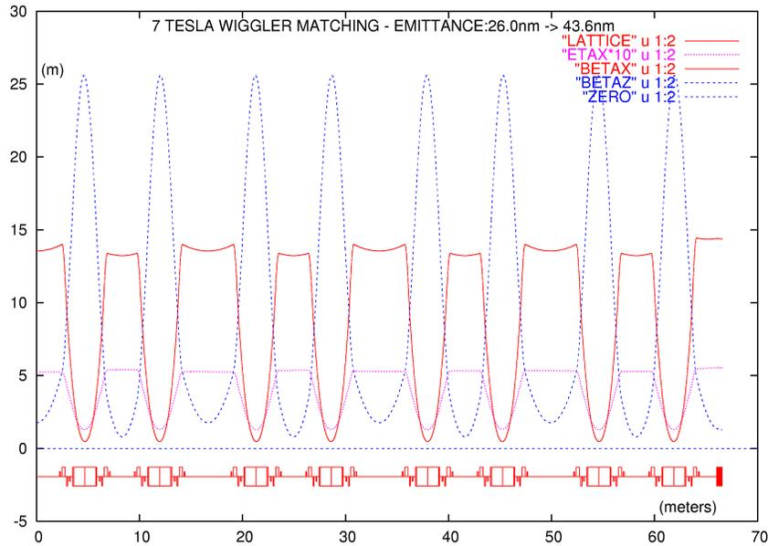
Figure 4: Half ring optical functions: the wiggler (1/2) is the last element of the lattice.
