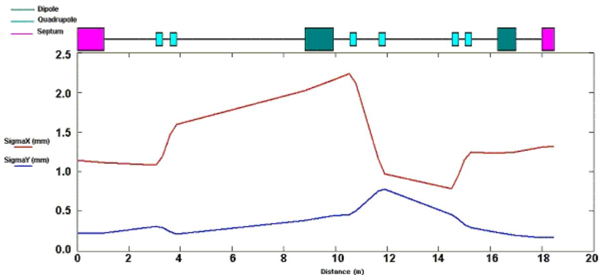
Figure 11.7: Horizontal and Vertical beam half width, and its variation in the transfer line for full match.
