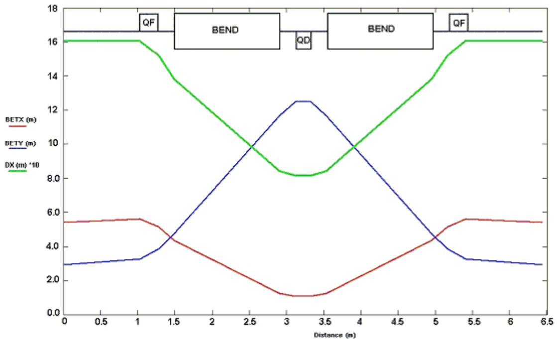
Figure 11.4: Beta functions and Horizontal Dispersion function versus position in one cell of the booster synchrotron consisting of two bending magnets and three quadrupoles.
