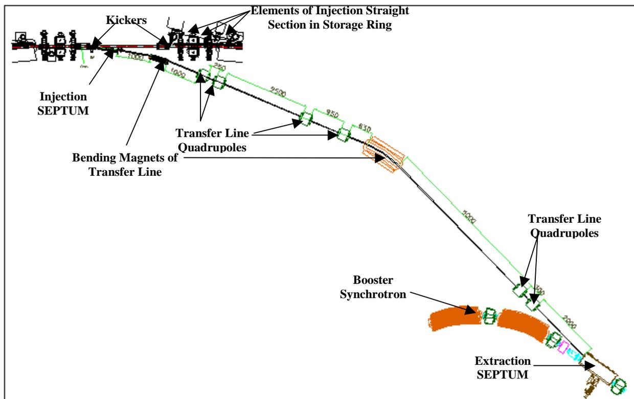
Figure 11.8: The transfer line and its elements and their arrangement with respect to the booster and the storage ring.
