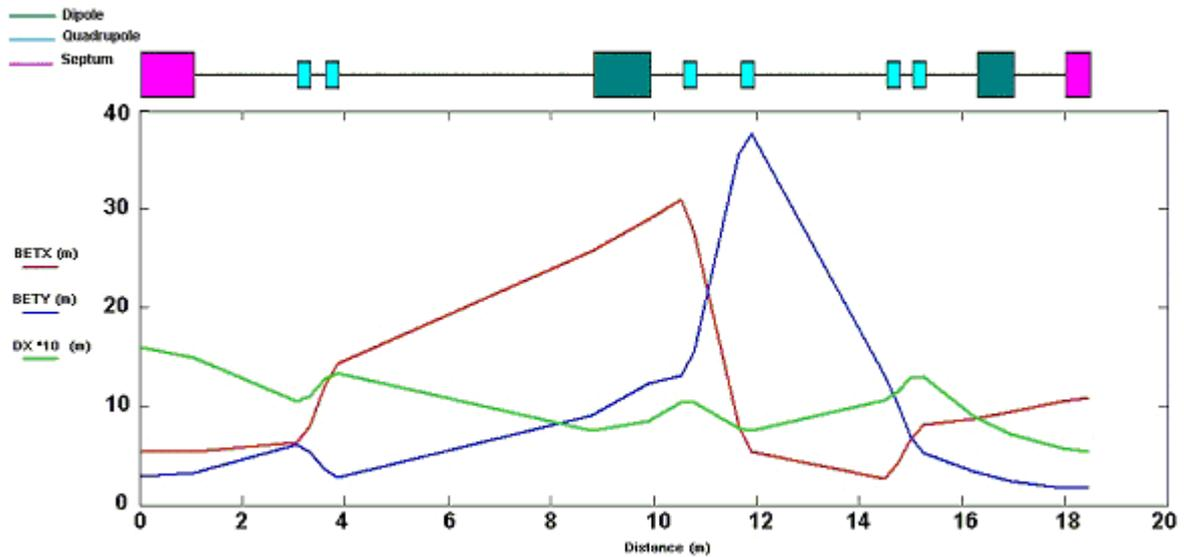
Figure 11.6: Main optical functions versus position in the transfer line for full matching.
