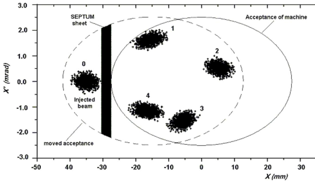
Figure 11.12: Injected beam and its movement in phase space at the injection point during the action of kickers.
