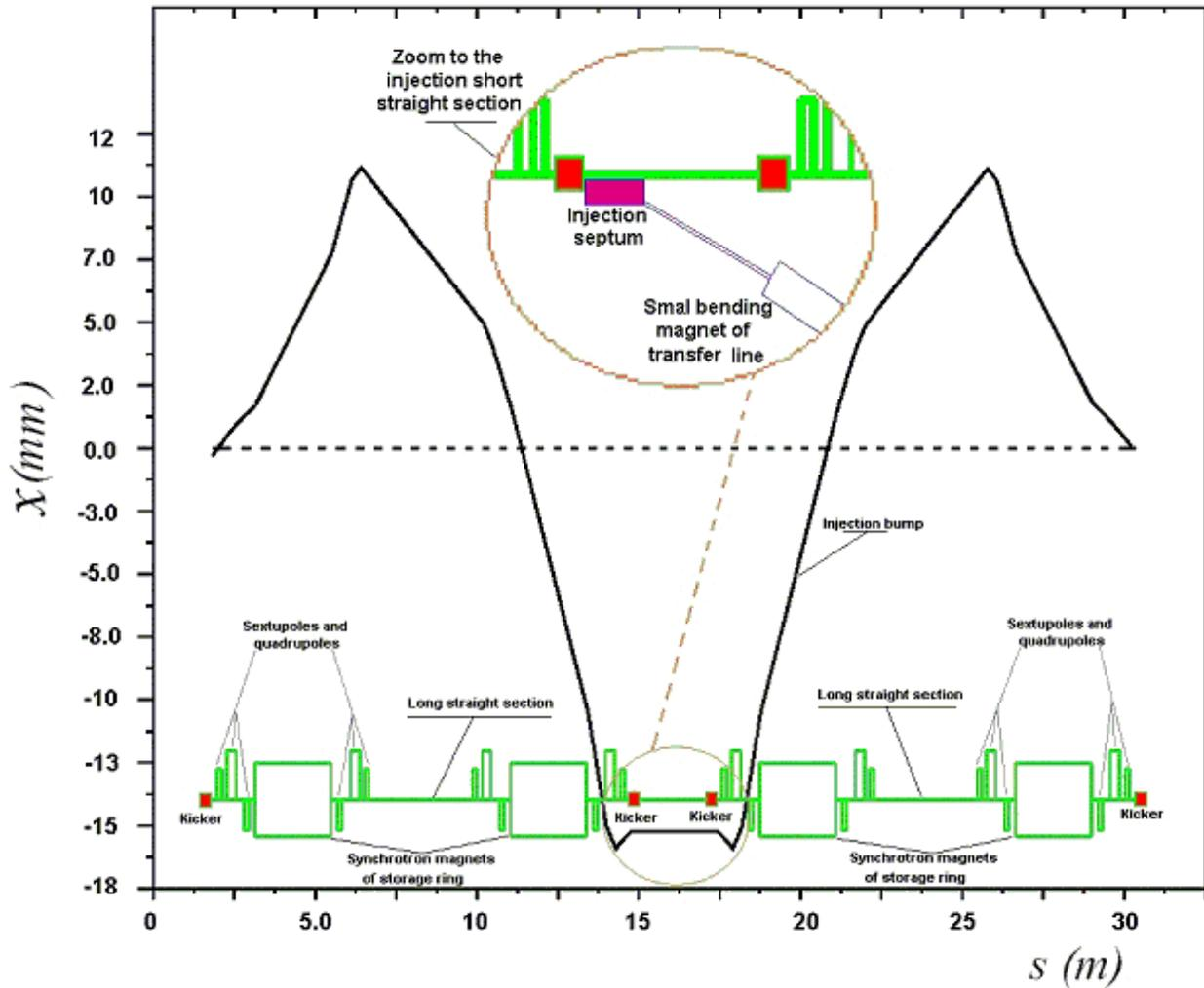
Figure 11.9: Layout of the injection region of SESAME showing also the orbit bump by means of four kickers.
