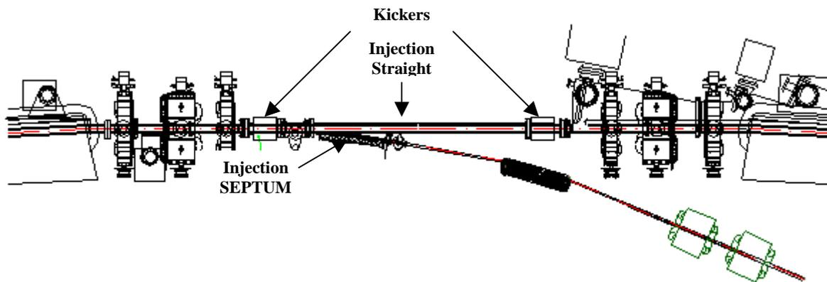
Figure 11.10: the layout of the injection straight.
