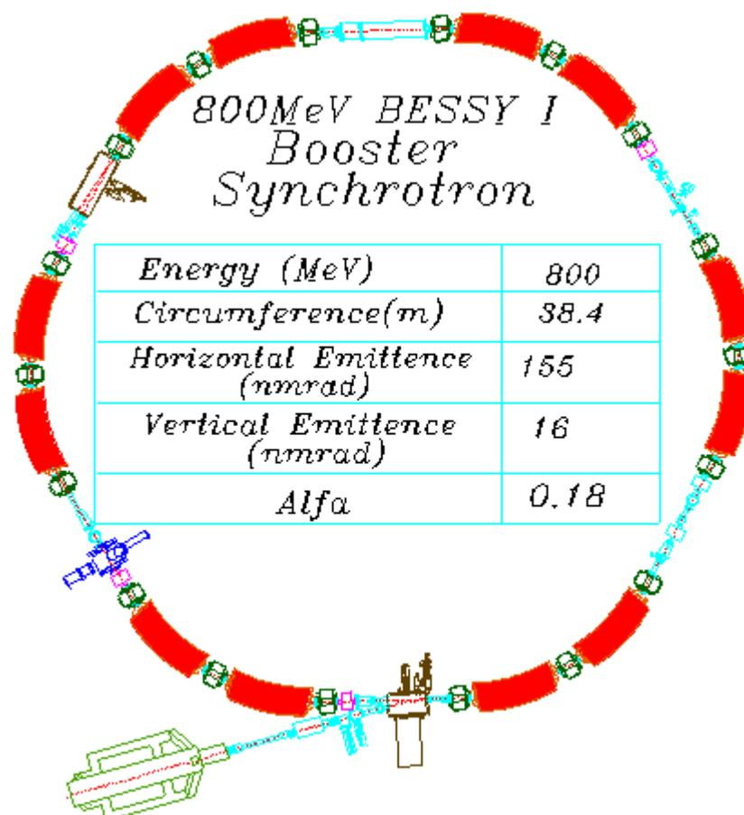
**Figure 11.2: Layout of the booster synchrotron and the microtron.**
