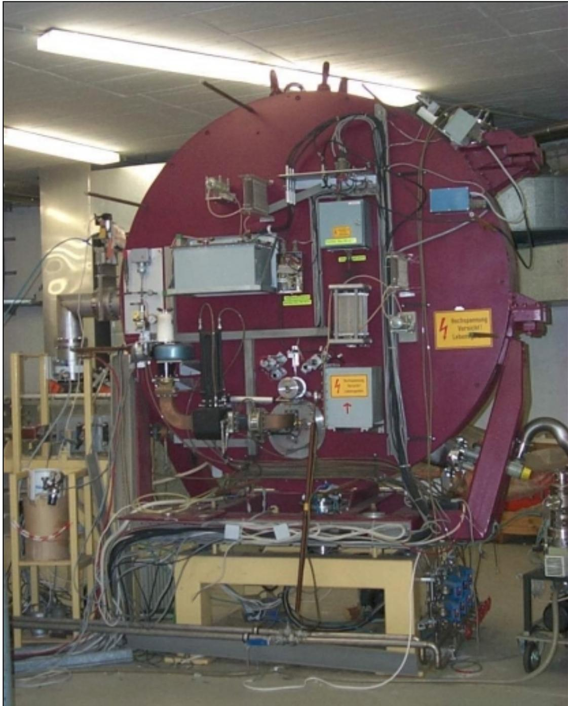
Figure 11.1: Microtron of BESSY I during disassembly.
