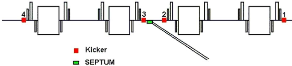
Figure 11.11: Three high beta sections of the storage ring with two low beta sections in between. Kickers are placed in high beta sections
