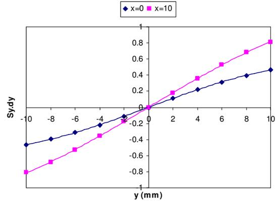
Figure 7: bpm sensitivity curves for y direction.
