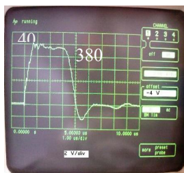
Figure 2: The modulator pulse current that we measured (left) compared to the one measured at BESSY I in 1998(right).
