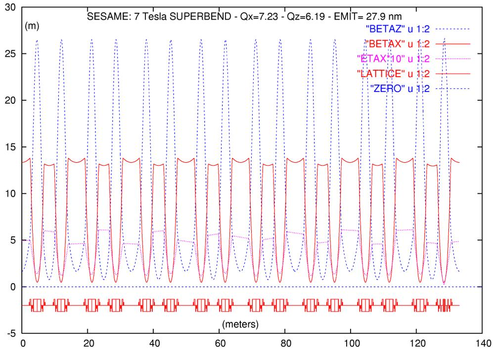
Figure 5: SESAME full ring optical function for the SUPERBEND solution.
