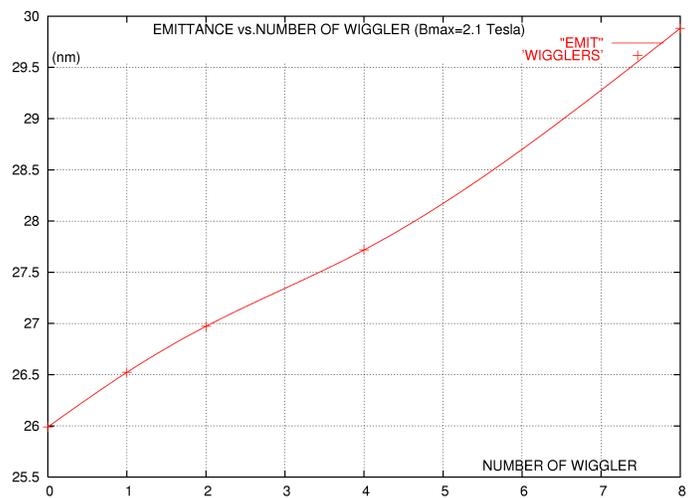
Figure 3: Emittance vs. the number of 23-period wigglers (the max number is obviously 8).
