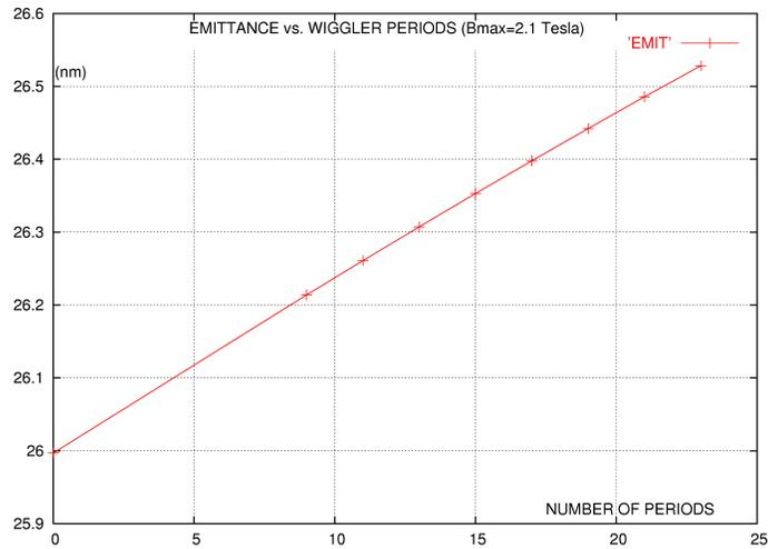
Figure 2: Emittance vs. the number of wiggler periods.
