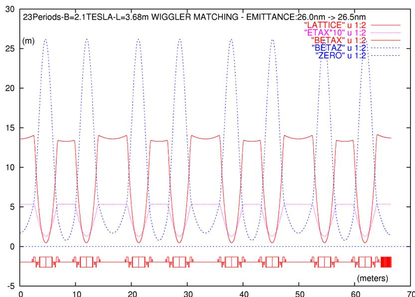
Figure 1: Half ring optical functions: the wiggler (1/2) is the last element of the lattice.
