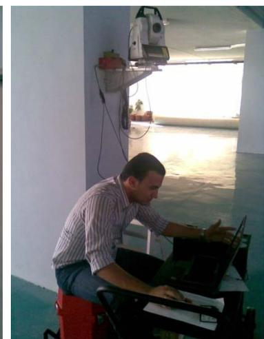
A short checking of the network was held on 30th October 2009; 4 wall brackets were measured again in order to compare with the initial survey. The corresponding meteorological correction has been applied to the distance measurements. A linear tendency appears in the distances comparison of about  $10^{-5}$ . That error may come from meteorological uncertainty. However, the control of the network size is enough at this level of precision.
