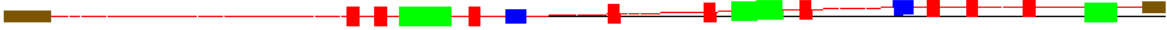
Figure 6: Transfer line layout (Auto Cad drawing) showing septums (brown), quadrupoles (red), horizontal bendings (green) and vertical bendings (blue). The final elevation is 20cm from zero level. (plotted by A. Amro).
