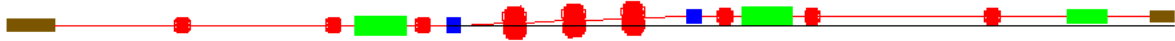
Figure 10: Transfer line drawing showing extraction and injection septums (brown), quadrupoles (red), horizontal bendings (green) and vertical bendings (blue). The final elevation is 20cm from zero level. (plotted by A. Amro).
