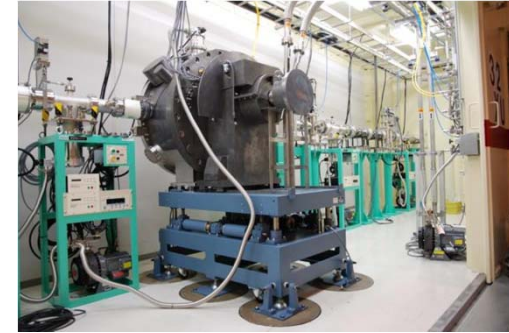
High precision double crystal monochromator
