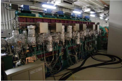
Hybrid in-vacuum undulator
