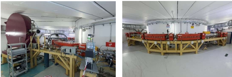
Fig 1.7: Microtron and transfer line TL1 (left), and booster (right).
