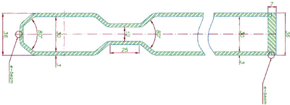
Figure 5.9: Cross section of the dipole vacuum chamber
