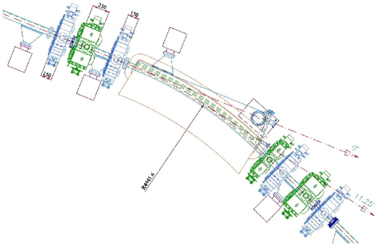
**Figure 5.5: Top view of the dipole vacuum chamber, 2nd dipole of the super period**
