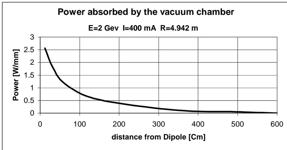
**Figure 5.16: Power absorbed by the distributed absorber in the vacuum chamber**
