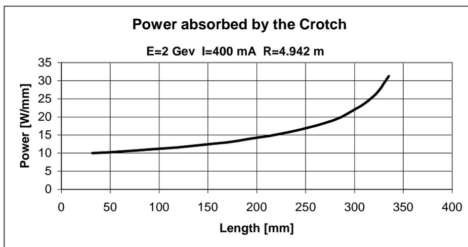
Figure 5.13: Power absorbed by the crotch in the dipole
