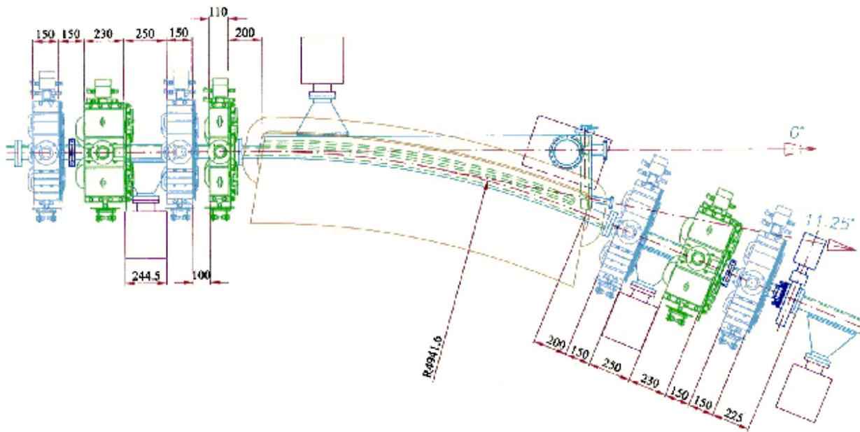
Figure 5.4: Top view of the dipole vacuum chamber, first dipole of the super period
