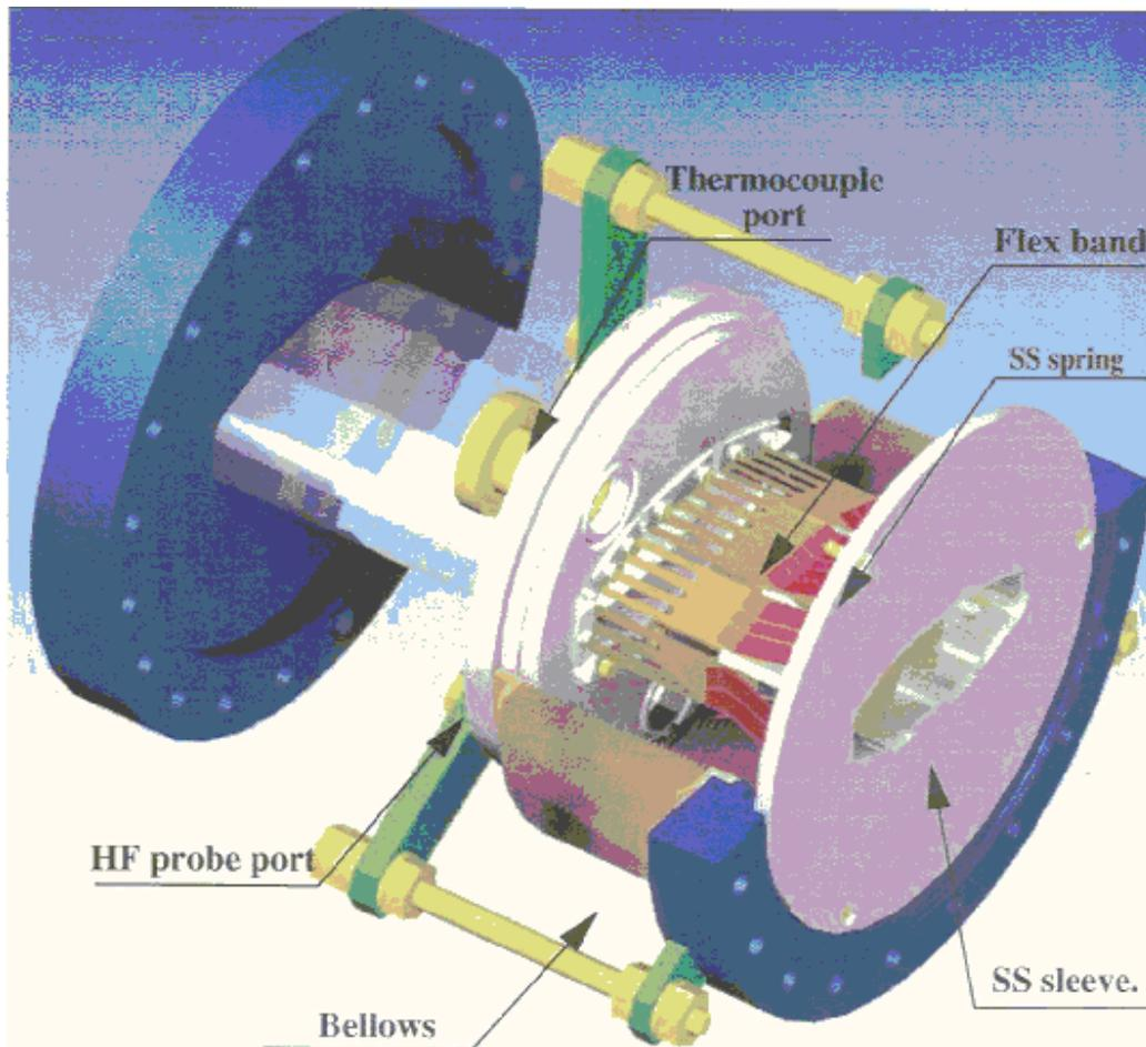
Figure 5.10: Schematic view of an RF shielded bellows
