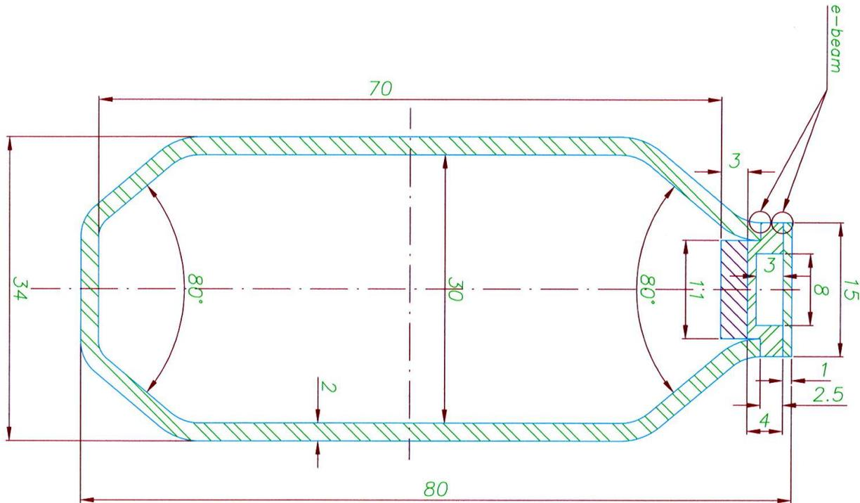
Figure 5.8: Cross section of the multipole vacuum chamber
