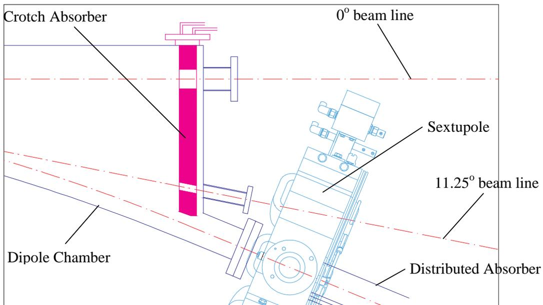
Figure 5.12: The crotch absorber on the dipole magnet
