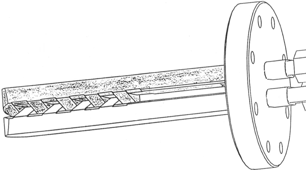
**Figure 5.15: An overall view of the crotch absorber**
