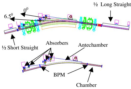
Figure 8: The unit half-cell of the storage ring.
