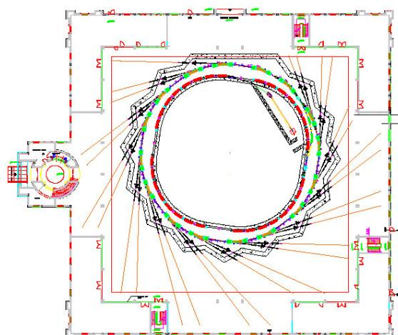
Figure 3: SESAME layout with full-energy injector.
