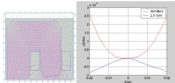
Figure 9: Dipole cross section and transverse field quality within  $\pm 2$  cm at 2.5 GeV and 800 MeV.
