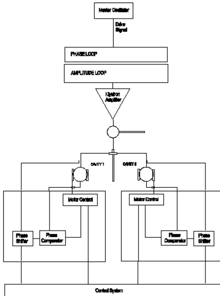
Figure 8.11: Tuning loop scheme.
