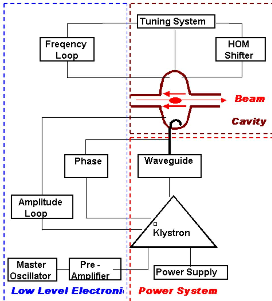
Figure 8.2: A schematic layout of the RF system for a synchrotron light source. The main groups of the system are the cavities, the power system and the low level electronics.
