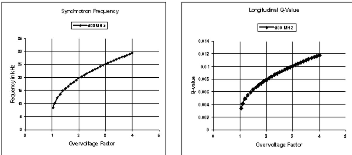
Figure 8.6: Synchrotron frequency and longitudinal working point of SESAME as a function of the over voltage factor for an energy of 2 GeV.
