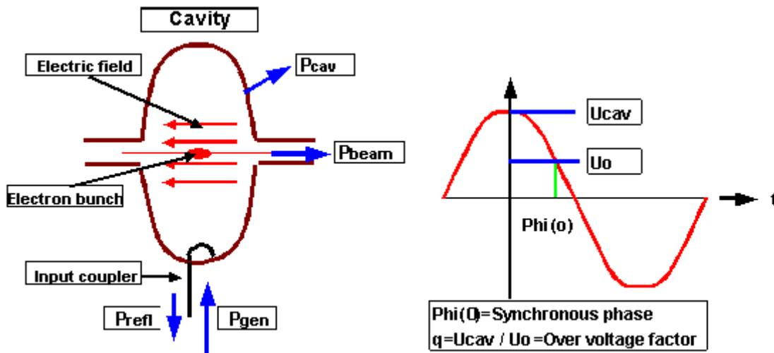
Figure 8.4: Schematic drawings for the explanations of used expressions for the RF system
