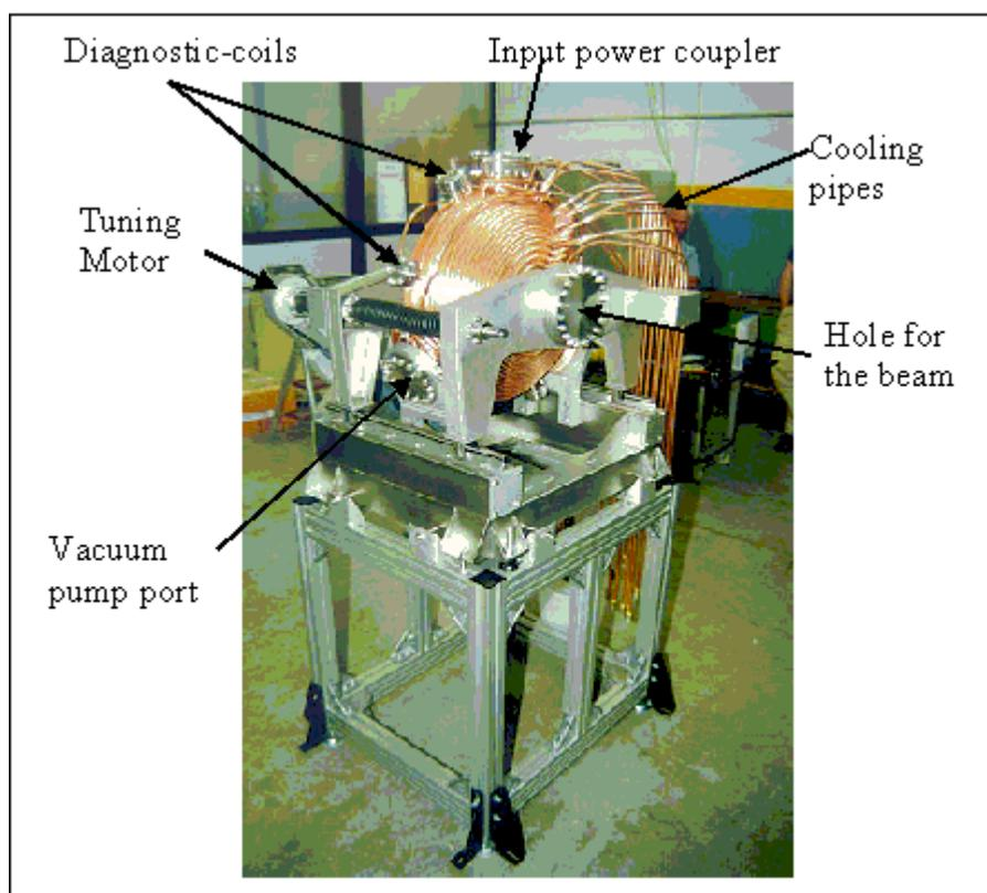
Figure 8.3: Cavity and their parts.
