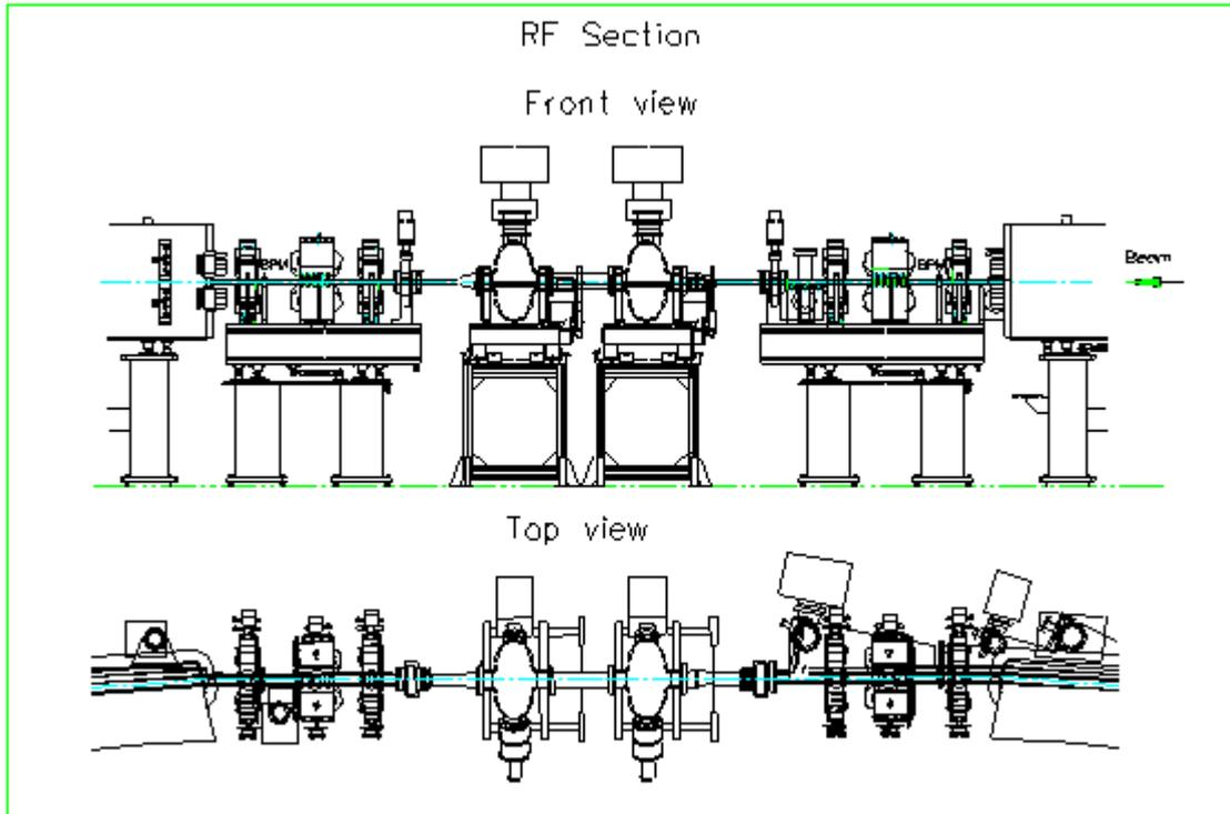
Figure 8.7: Arrangement of 2 cavities in the long straight section of SESAME.
