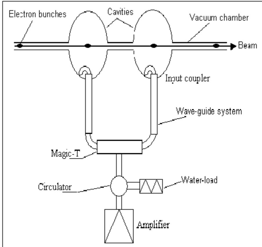
**Figure 8.8: RF-power assembly layout at the first stage with 2 cavities and an power of the amplifier of up to 250 kW in order to operate SESAME at an energy of 2 GeV with 2 wigglers or 2.5 GeV without any wigglers. This is the “RF-unit” of SESAME**
